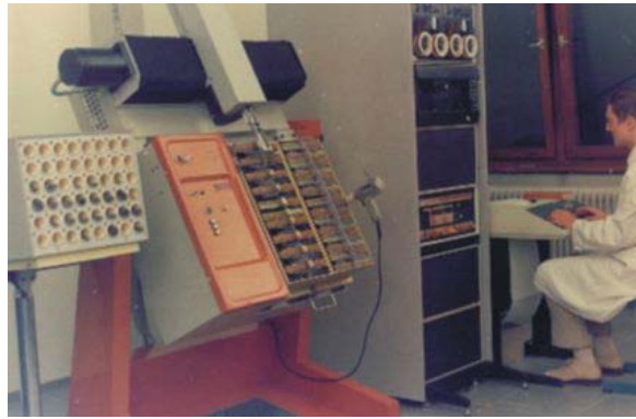
Fig. 5. Computer controlled system for the wiring of telephone exchanges (personal archive).
