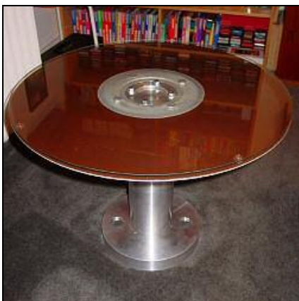
Fig.10: The hard disk 6603 of the Control Data Corporation (1967). The diameter was 66 cm and the capacity of 512 Kb. Here it has been transformed into a table
